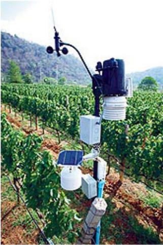
Weather sensors monitor humidity, temperature, mass movement of the air, rain accumulation and sunlight energy in vineyards.
